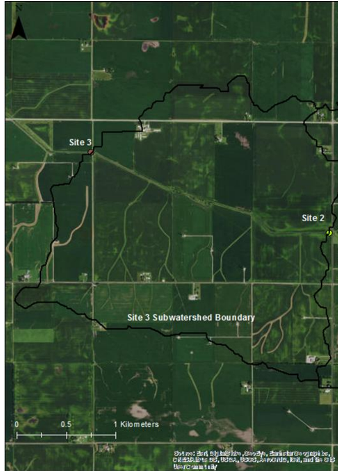
Figure 61. An Aerial image showing the site 3 subwatershed and the western border of the Site 2 subwatershed. The creek flows from east to west. Notice that the total area of fields that exist both within and outside of the Site 3 watershed is limited.
